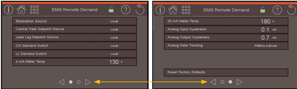
Figure 16: Remote Demand Setup Screens
