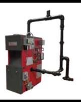
The near boiler piping kit will assist in delivering "dry" steam to the heating system, reduce short cycling, eliminate water hammering and protect against system flooding. Kit includes all components required to complete the near boiler piping as recommended in the installation manual.
